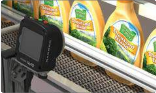
Label detection using a Match Sensor
