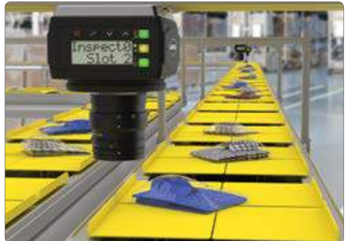
Empty sortation conveyor inspection using Blemish Tool
