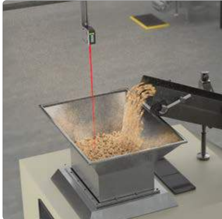
Monitoring levels inside a high-volume hopper
