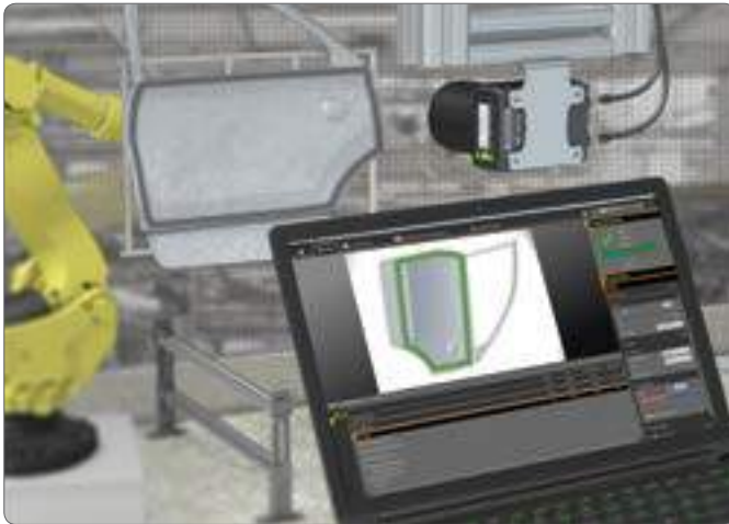
Door panel adhesive inspection using Bead Tool
