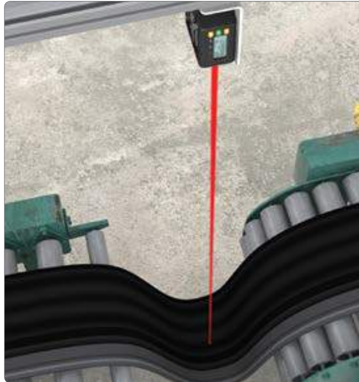
Loop control on a calendering machine
