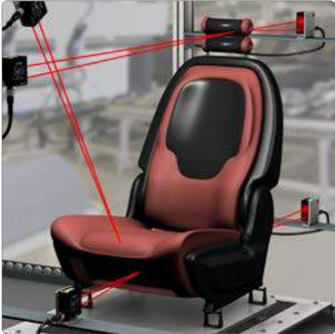
Auto seat adjustment measurement using the LE550
