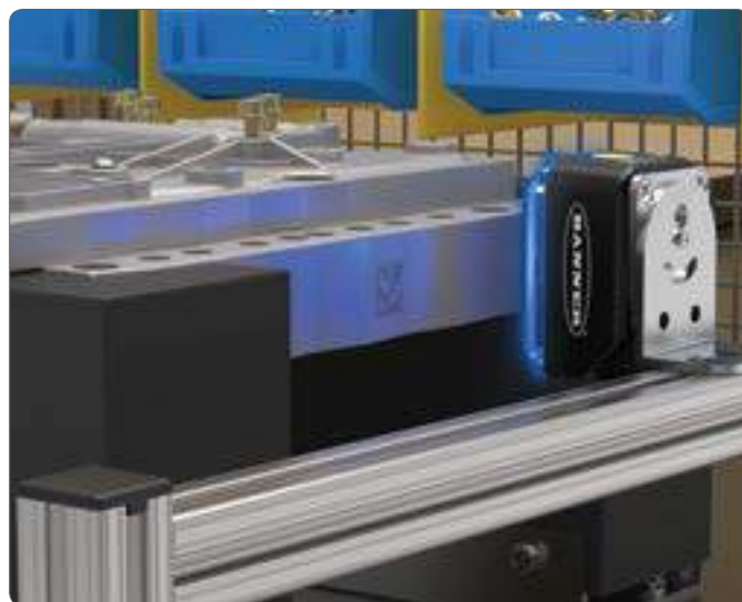
Direct Part Mark (DPM) code reading and verification on automotive part
