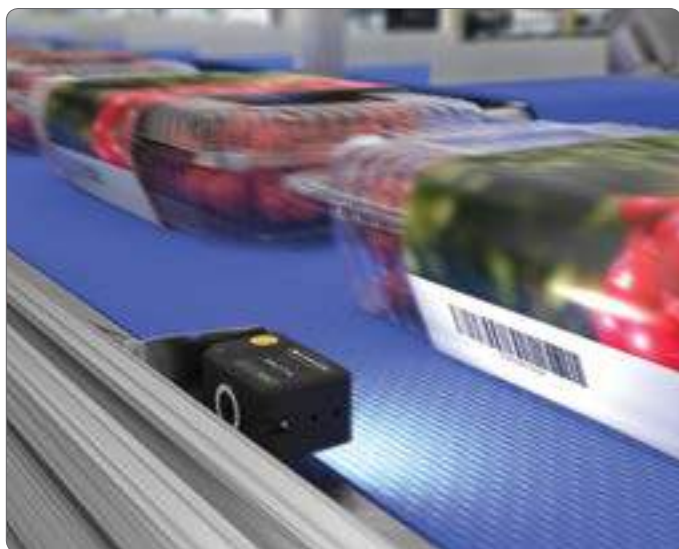
Barcode reading for food traceability
