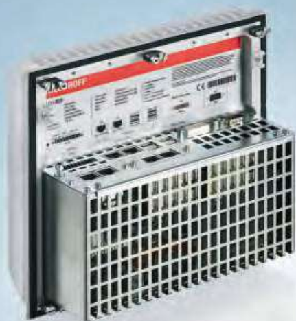
C6515 with PCIe module slots
