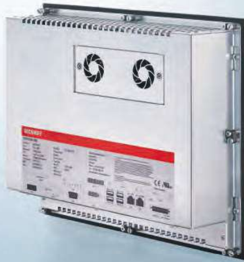
CP62xx with PCIe module slots C9900-B500
