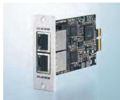
PCIe module FC9062, dual gigabit Ethernet
