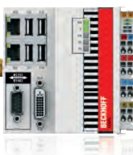
CX5020 with D-sub plug, 9-pin
