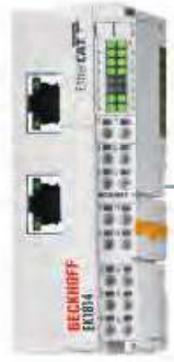
EtherCAT Coupler with integrated digital I/Os
