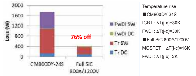
Figure 11: Loss and \Delta T(j-c) simulation at f_c=30\text{kHz}; V_{CC}=600\text{V}; I_O=400\text{A(peak)}; PF=0,8; M=1,0
