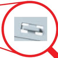
By breaking off the protruding ribs (by hand), the separator becomes only 1.8 mm thick; useful for the visual separation of different groups of interfaces, or necessary for the protective separation of different voltages of neighbouring interfaces, or for the protection of cut ends of jumper links.
