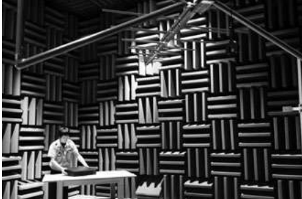
Acoustic radio wave anechoic chamber
