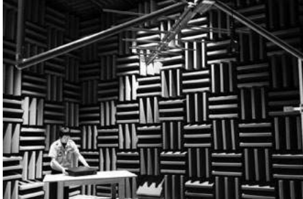
Acoustic radio wave anechoic chamber
