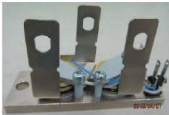
Pressure contact design – no wire bonds, no solder fixation
