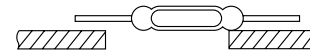
Fig. 7 Precautions to be taken when mounting reed switch on printed wiring board
