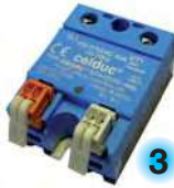
SO4 housing with different control connections.
